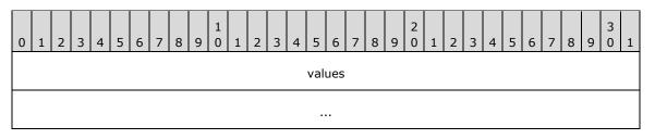
**values (8 bytes):** The set of values, each occupying 4 bits, in sequence and ordered low to high. In the sequence, the first value occupies Bits 0 through 3, the second value occupies Bits 4 through 7, and so on.
