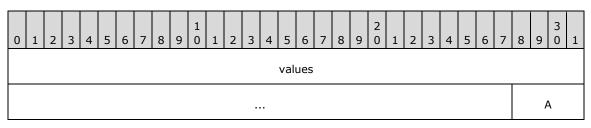
**values (60 bits):** The set of values, each occupying 6 bits, in sequence and ordered low to high. In the sequence, the first value occupies Bits 0 through 5, the second value occupies Bits 6 through 11, and so on.
