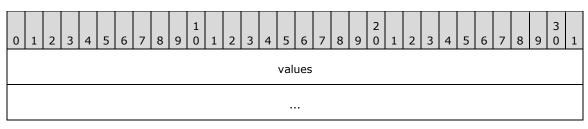
values (8 bytes): The set of values, each occupying 2 bits, in sequence and ordered low to high. In the sequence, the first value occupies Bits 0 through 1, the second value occupies Bits 2 through 3, and so on.
