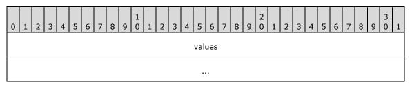
**values (8 bytes):** The set of values, each occupying 1 byte, in sequence and ordered low to high. In the sequence, the first value occupies Bits 0 through 7, the second value occupies Bits 8 through 15, and so on.
