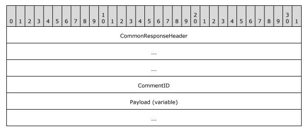
**CommonResponseHeader (12 bytes):** This is the **Common Response** header, as specified in section 3.1.4.1.1.
