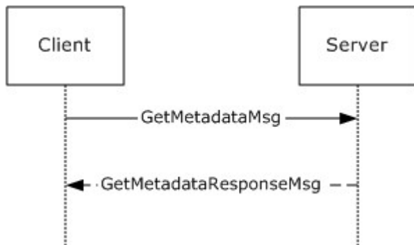
Figure 1: Message pattern of the User Profile Synchronization (UPS): Schema Exchange Protocol Profile
