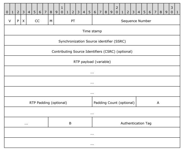
V, P, X, CC, M, PT, Sequence Number, Time stamp, SSRC, CSRC, RTP payload, RTP Padding, Padding Count: Standard RTP packet fields. For details, see [RFC3550] section 5.1.
