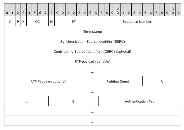
V, P, X, CC, M, PT, Sequence Number, Time stamp, SSRC, CSRC, RTP payload, RTP Padding, Padding Count: Standard RTP packet fields. For details, see [RFC3550] section 5.1.
