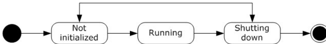
Figure 2: State machine diagram for the protocol server
