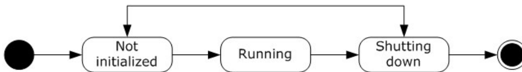
Figure 2: State machine diagram for the protocol server
