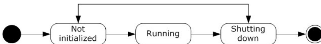
Figure 2: State machine diagram for the protocol server
