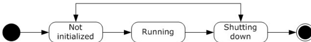
Figure 2: State machine diagram for the protocol server
