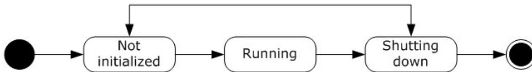
Figure 2: State machine diagram for the protocol server
