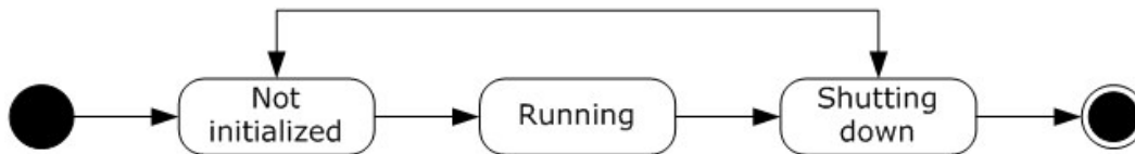
Figure 2: State machine diagram for the protocol server
