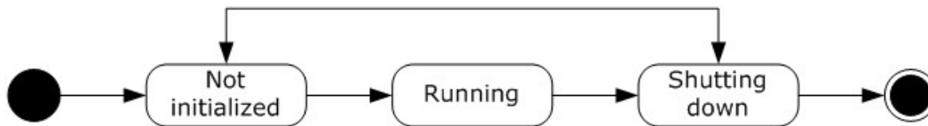
Figure 2: State machine diagram for the protocol server
