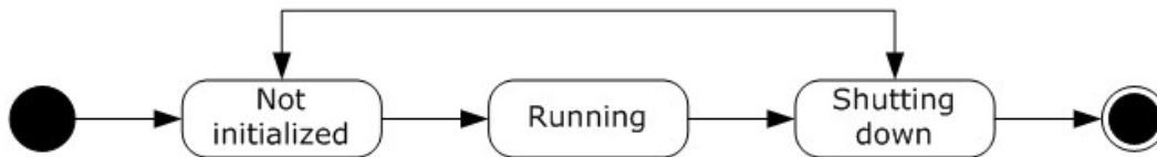
Figure 2: State machine diagram for the protocol server
