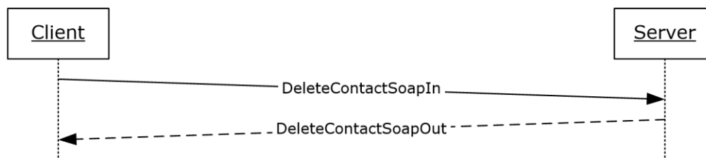
Figure 7: Message sequence for a DeleteContact operation
