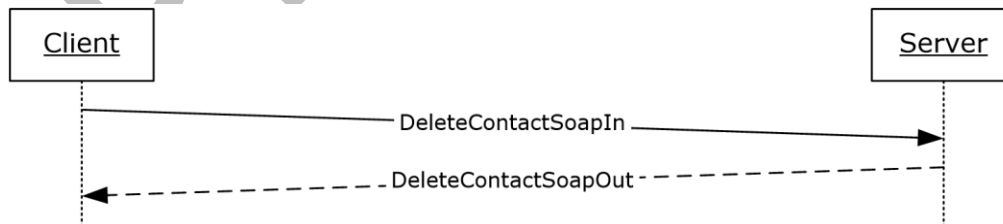
Figure 7: Message sequence for a DeleteContact operation
