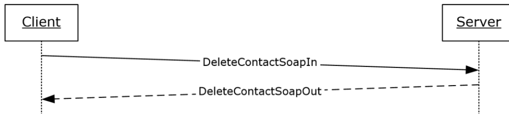
Figure 7: Message sequence for a DeleteContact operation
