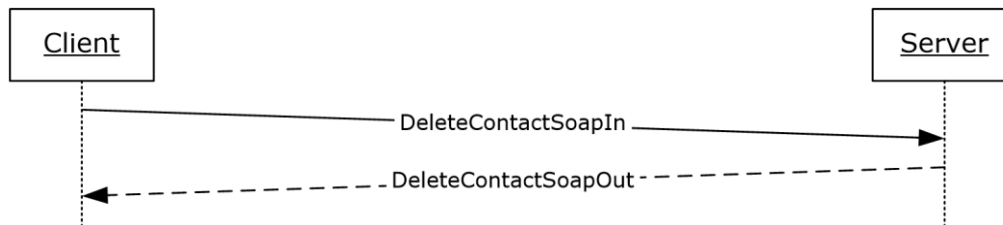
Figure 7: Message sequence for a DeleteContact operation
