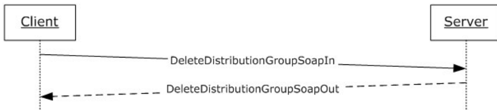
Figure 8: Message sequence for a DeleteDistributionGroup operation
