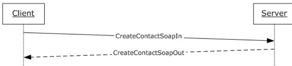
Figure 5: Message sequence for a CreateContact operation
