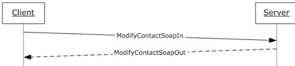
Figure 10: Message sequence for a ModifyContact operation
