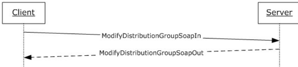
Figure 11: Message sequence for a ModifyDistributionGroup operation
