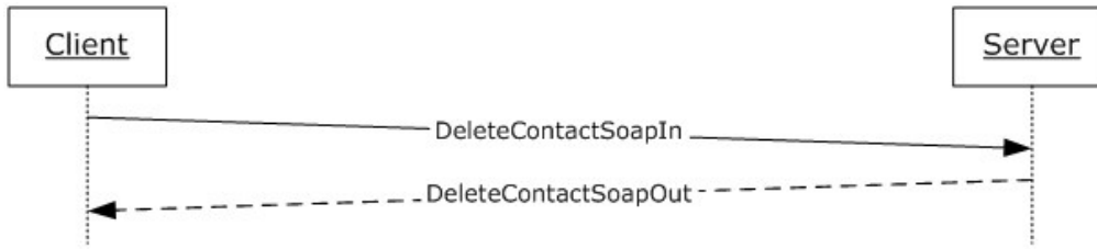
Figure 7: Message sequence for a DeleteContact operation
