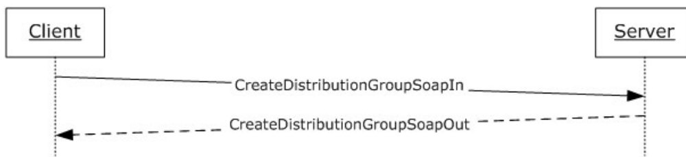
Figure 6: Message sequence for a CreateDistributionGroup operation
