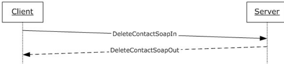
Figure 7: Message sequence for a DeleteContact operation
