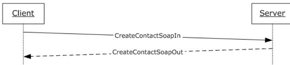
Figure 5: Message sequence for a CreateContact operation
