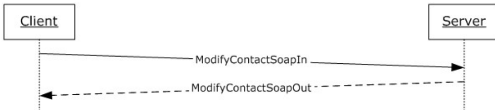
Figure 10: Message sequence for a ModifyContact operation
