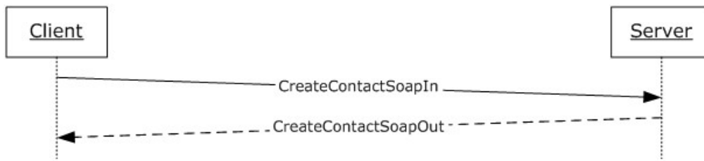
Figure 5: Message sequence for a CreateContact operation
