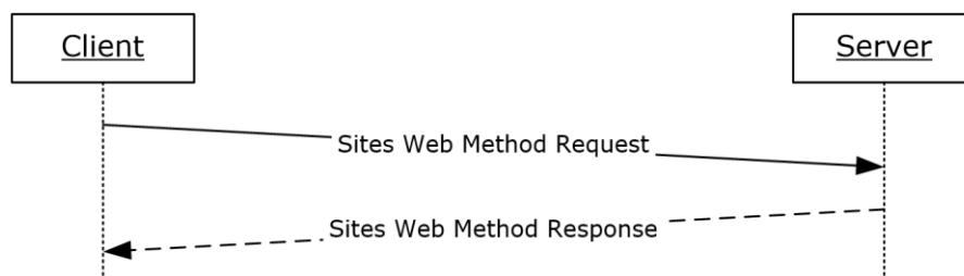
Figure 1: Sites Web method sequence diagram
