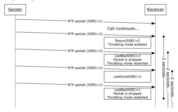
Figure 5: Synchronization source change throttling
