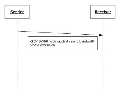
Figure 21: Message Exchange for Modality Send Bandwidth Limit Extension
