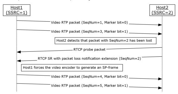
Figure 10: Message exchange for packet loss notifications
