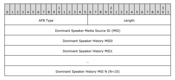
**AFB Type (2 bytes):** The application layer feedback message type. Set to 0x3.
