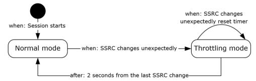
Figure 2: Synchronization source throttling
