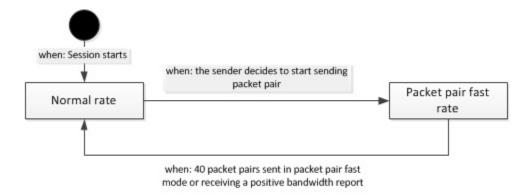
Figure 3: Behavior of packet pair bandwidth acceleration
