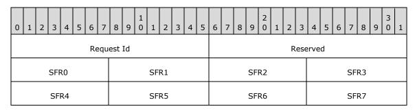
**Request Id (2 bytes):** A 16-bit unsigned number that uniquely identifies the PLI. A PLI may be sent multiple times to improve redundancy. All the retransmitted PLIs MUST carry the same Request Id. A different PLI MUST carry a different Request Id.
