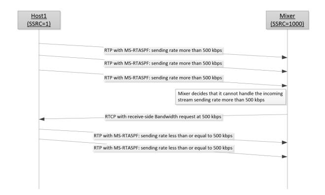
Figure 15: Message exchange for receiver-side bandwidth limit
