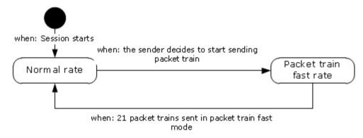
Figure 4: Behavior of packet train bandwidth acceleration
