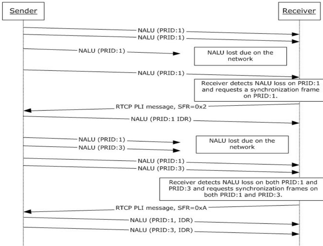
**Figure 18: Picture Loss Indication Extension**
