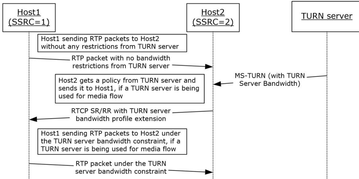
**Figure 13: Message exchange for TURN Server bandwidth extension**
