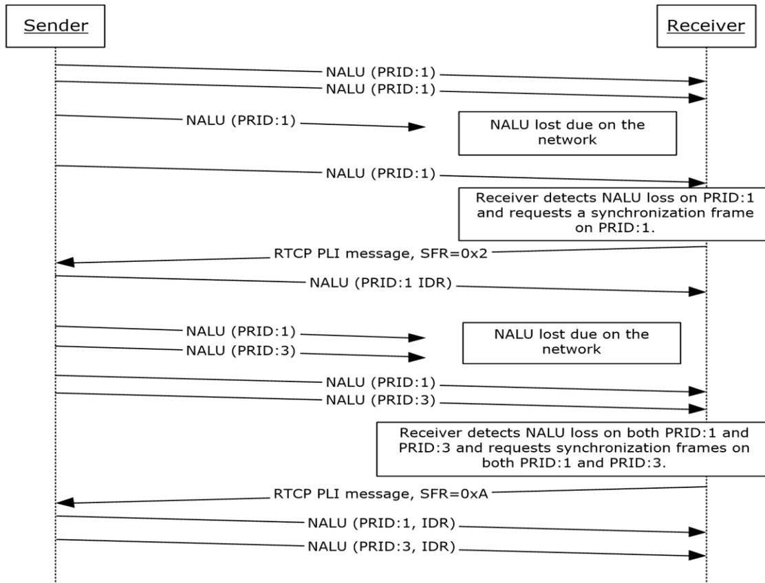
**Figure 18: Picture Loss Indication Extension**
