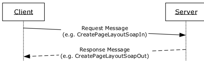
Figure 2: Sequence diagram showing the typical message pattern
