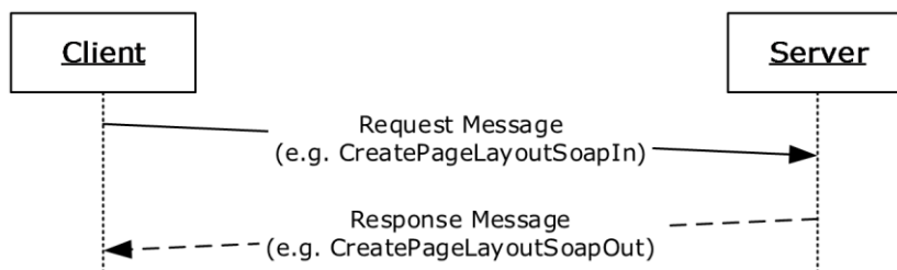
Figure 2: Sequence diagram showing the typical message pattern
