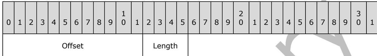
**Offset (12 bits):** This field contains an index from the beginning of the dictionary that indicates where the matched content will start.
