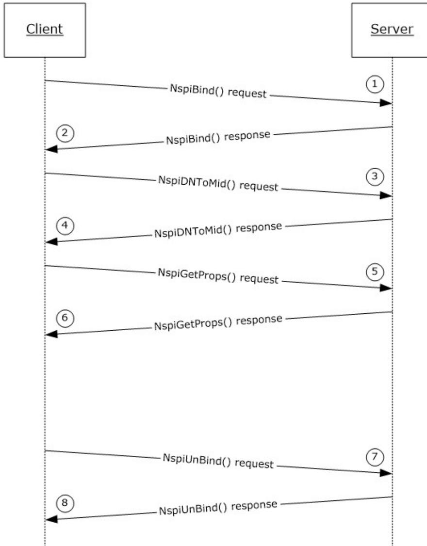
**Figure 1: Call sequence between client and server**
