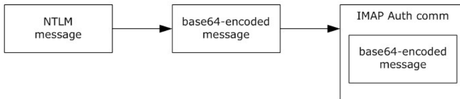
Figure 1: Relationship between NTLM message and IMAP4: NTLM Authentication Protocol message
