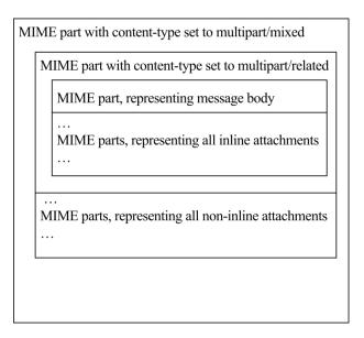
Figure 1: Inline and non-inline attachments present
