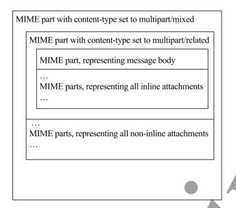
Figure 1 Inline and non-inline attachments present
