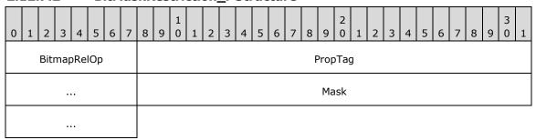
**BitmapRelOp (1 byte):** This value encodes the **BitmapRelop** field of the **BitMaskRestriction** structure, as specified in section 2.12.7.1.
