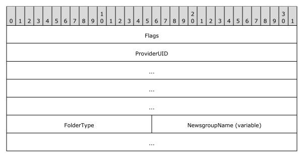
**Flags (4 bytes):** This value MUST be set to 0x00000000. Bits in this field indicate under what circumstances a short-term **EntryID** is valid. However, in any EntryID stored in a property value, these 4 bytes MUST be zero indicating a long-term EntryID.
