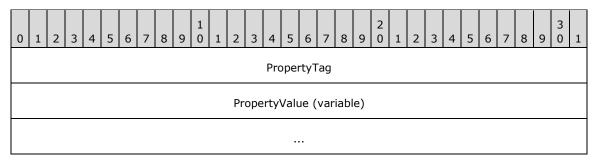
**PropertyTag (4 bytes):** A **PropertyTag** structure, as specified in section <u>2.9</u>, giving the values of the **PropertyId** and **PropertyType** fields for the property.
