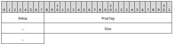
**Relop (1 byte):** This value encodes the **Relop** field of the **SizeRestriction** structure, as specified in section 2.12.8.1.
