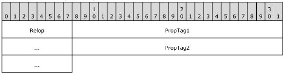
**Relop (1 byte):** This value encodes the **Relop** field of the **ComparePropertiesRestriction** structure, as specified in section 2.12.6.1.
