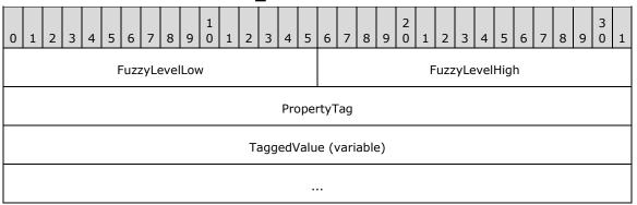
**FuzzyLevelLow (2 bytes):** This value encodes the **FuzzyLevelLow** field of the **ContentRestriction** structure, as specified in section 2.12.4.1.
