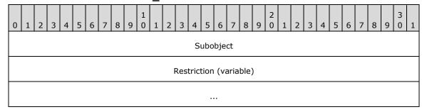
**Subobject (4 bytes):** This value encodes the **Subobject** field of the **SubObjectRestriction** structure, as specified in section 2.12.10.1.
