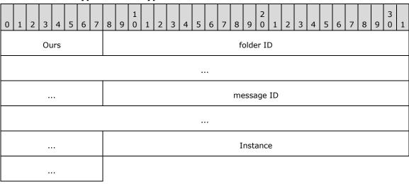
**Ours (1 byte):** The value 0x01 indicates the remaining bytes conform to this structure; the value 0x00 indicates this is a client-defined value and has whatever size and structure the client has defined.
