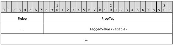
**Relop (1 byte):** This value encodes the **Relop** field of the **PropertyRestriction** structure, as specified in section 2.12.5.1.
