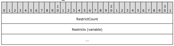
**RestrictCount (4 bytes):** Encodes the **RestrictCount** field of the **AndRestriction** structure, as specified in section <u>2.12.1.1</u>. This value MUST NOT exceed 100,000.
