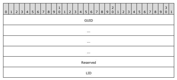
**GUID (16 bytes):** Encodes the GUID field of the **PropertyName** structure, as specified in section 2.6.1.
