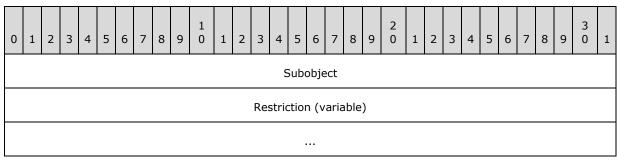
**Subobject (4 bytes):** Encodes the **subobject** field of the **SubObjectRestriction** structure. For more details, see section 2.12.10.1.
