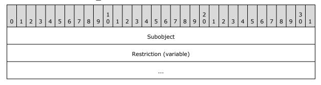
**Subobject (4 bytes):** Encodes the subobject field of the **SubObjectRestriction** structure. For more details, see section <u>2.12.10.1</u>.
