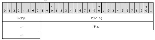
**Relop (1 byte):** Encodes the **Relop** field of the **SizeRestriction** structure. For more details, see section 2.12.8.1.
