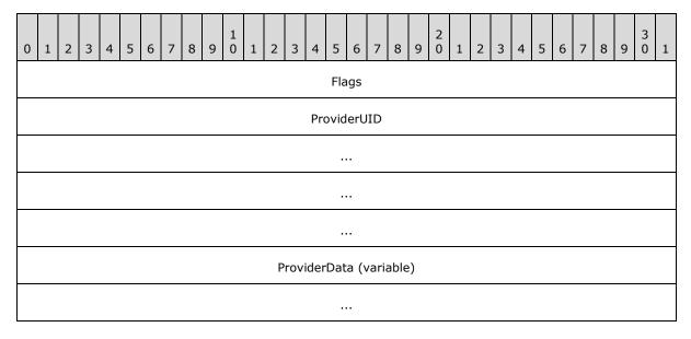
**Flags (4 bytes):** MUST be set to 0x00000000. Bits in this field indicate under what circumstances a short-term EntryID is valid. However, in any EntryID stored in a property value, these 4 bytes MUST be zero indicating a long-term EntryID.
