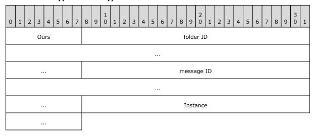
**Ours (1 byte):** 0x01 indicates the remaining bytes conform to this structure; 0x00 indicates this is a client-defined value, and has whatever size and structure the client has defined.
