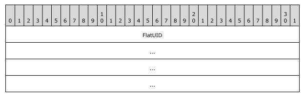
**FlatUID (16 bytes):** A flat 16-byte little-endian sequence used as a unique identifier in various structures.
