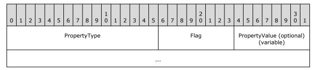
**PropertyType (2 bytes):** A 16-bit unsigned integer that specifies the data type of the property value, according to the table in section 2.11.1.
