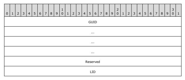
**GUID (16 bytes):** Encodes the GUID field of the **PropertyName** structure. For more details, see section 2.6.1.
