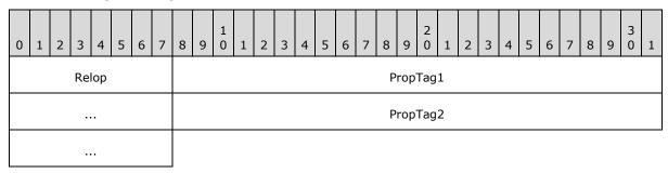
**Relop (1 byte):** Encodes the **Relop** field of the **ComparePropertiesRestriction** structure. For more details, see section 2.12.6.1.
