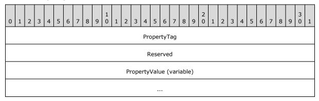
**PropertyTag (4 bytes):** Encodes the property tag with the value represented by the **PropertyValue\_r** structure.
