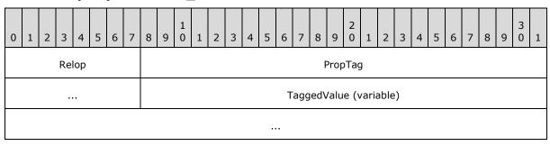
**Relop (1 byte):** Encodes the **Relop** field of the **PropertyRestriction** structure. For more details, see section 2.12.5.1.
