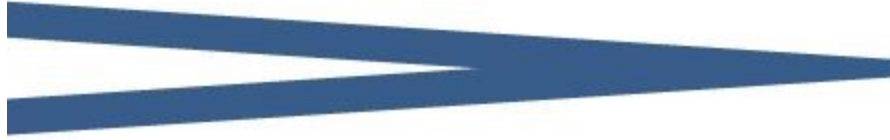
Figure 8: A line that was clipped because the miter length extended beyond the line miter limit
