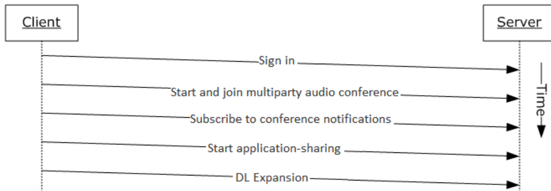
Figure 35: Sequence for starting a conference, joining with multiparty audio, and starting application-sharing, Distribution List (DL) Expansion
