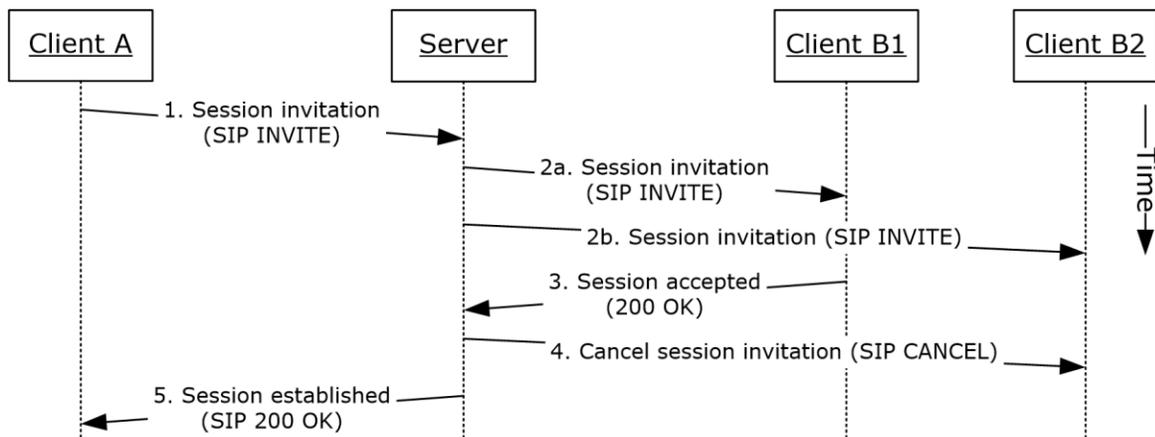
**Figure 15: Steps for using multiple endpoints (5)**
