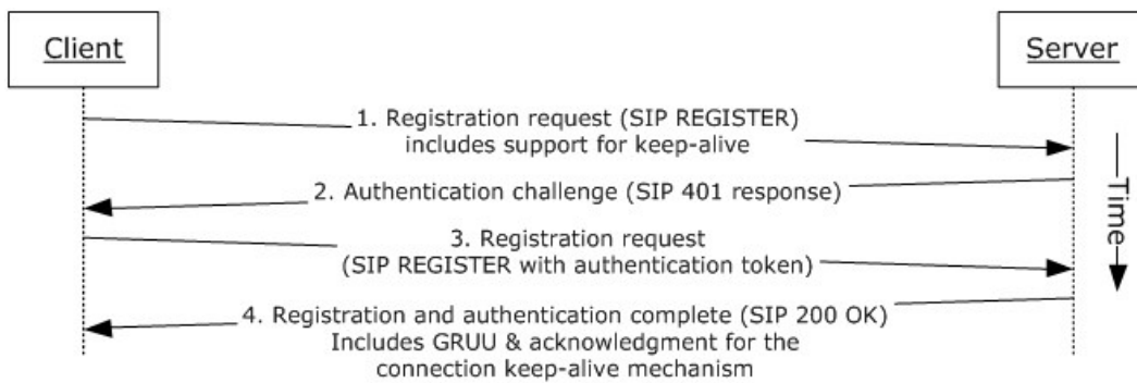
Figure 7: Steps for performing registration and authentication (2)
