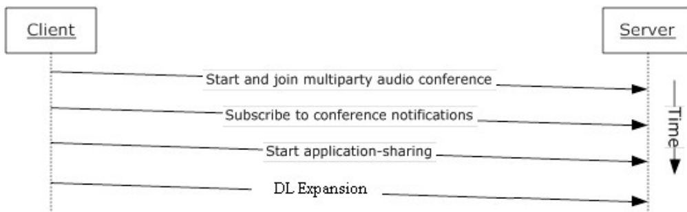
Figure 30: Sequence for starting a conference, joining with multiparty audio, and starting application-sharing, Distribution List (DL) Expansion
