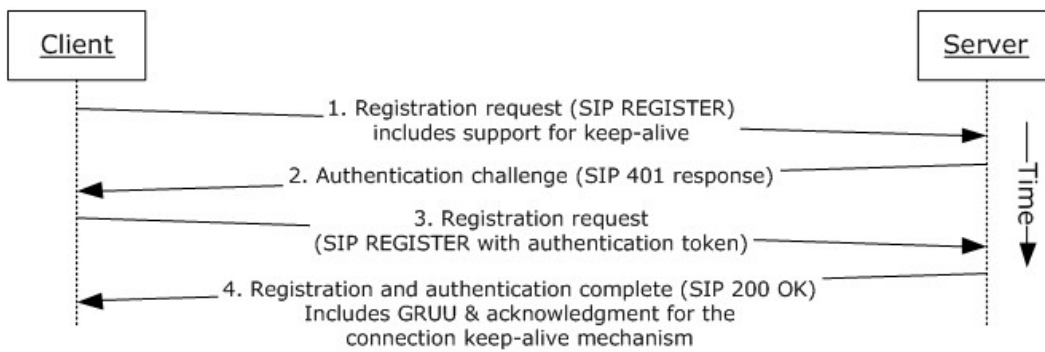
Figure 3: Steps for performing registration and authentication (2)
