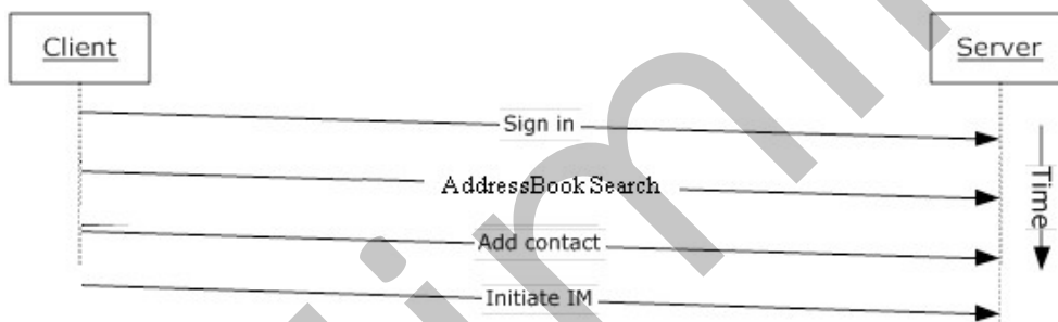
Figure 22: Sequence for sending an instant message to a contact
