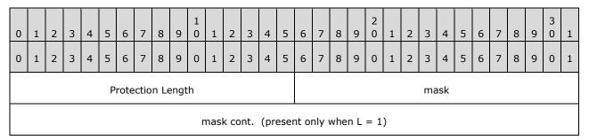
The protection length field and the mask field have the same meaning as defined in [RFC5109].
