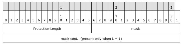
The protection length field and the mask field have the same meaning as defined in [RFC5109].
