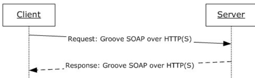
Figure 2: Message interaction between protocol client and protocol server
