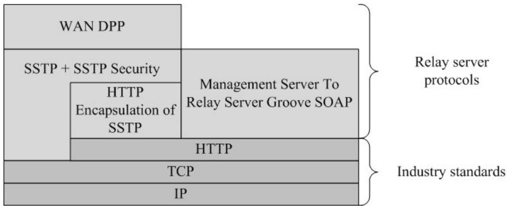
**Figure 7: Protocol stack for the relay server**
