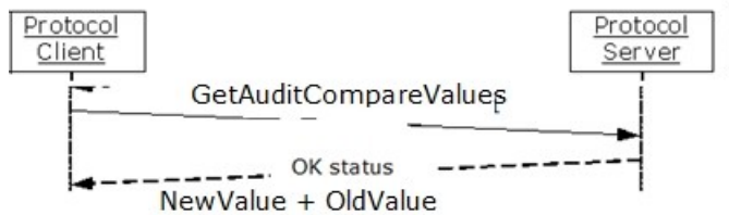
Figure 3: Communication sequence diagram for getting old and new values for comparison
